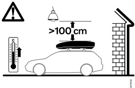
Be aware, that at least 100 cm is needed between the top of the roof box and the roof when parking inside.
