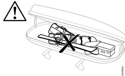
Always secure the load in the roof box with the supplied strap.
