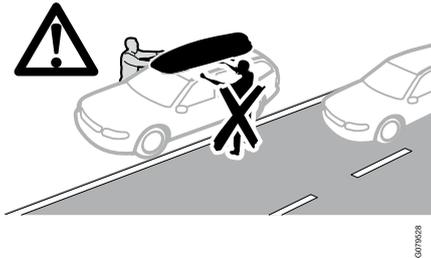
Always carefully approach the roof box near roads. Avoid approaching the roof box from the traffic side.
