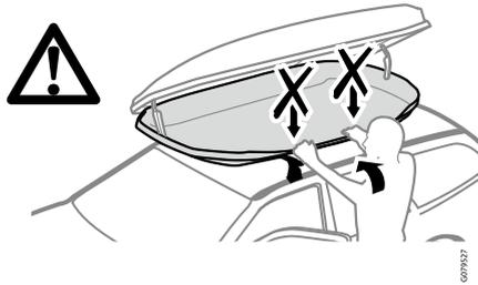
Avoid holding on the roof box rim as it may damage it.
