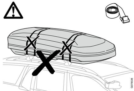
Never use straps to close the lid or to fix the roof box on the vehicle.
