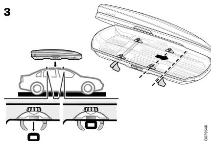
Make sure that the locking clamps are in place, and the roof racks are between the locking clamps.
