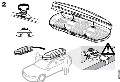
Loosen the 4 clamps counterclockwise
