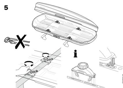
Make sure that the clamps are installed properly as illustrated
