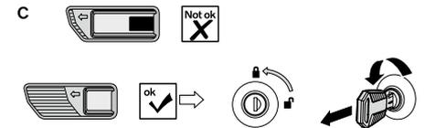
c, Make sure that the button is in the original position. Lock the roof box lid by turning the key counterclockwise, and remove the key.
