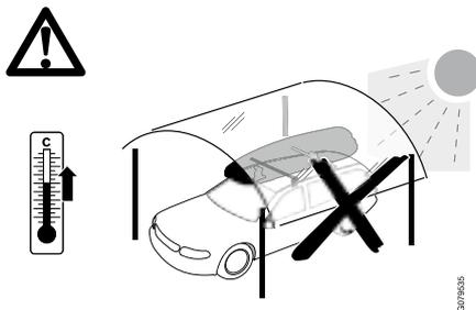
Never park under transparent roofed parking spots when the roof box is installed.
