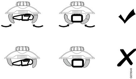
Make sure that the clamps holds the roof racks as illustrated.
