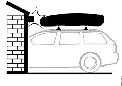
Be aware when parking in closed places that the roof box is on the roof of the vehicle and the total height is higher.
